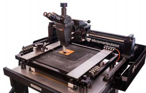
2210-LS System Level Prober with temperature stress
